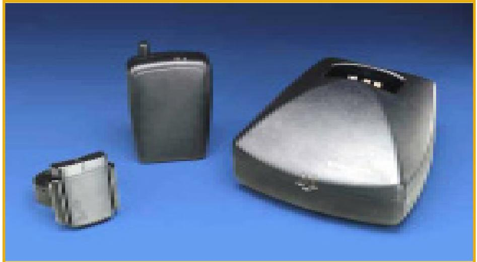
GPS monitoring is one tool used to assist with supervision of some ISR offenders. Pictured, from left to right, are the tracking unit worn by the offender, the transmitter carried by the offender, and the charging stand that downloads and transmits data.
