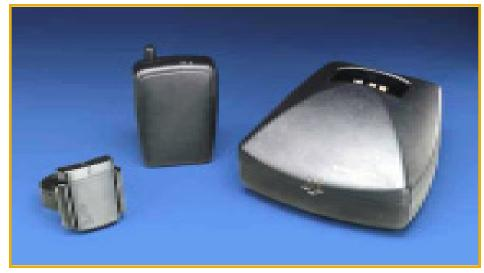
GPS monitoring is one tool used to assist with supervision of some ISR offenders. Pictured, from left to right, are the tracking unit worn by the offender, the transmitter carried by the offender, and the charging stand that downloads and transmits data.
